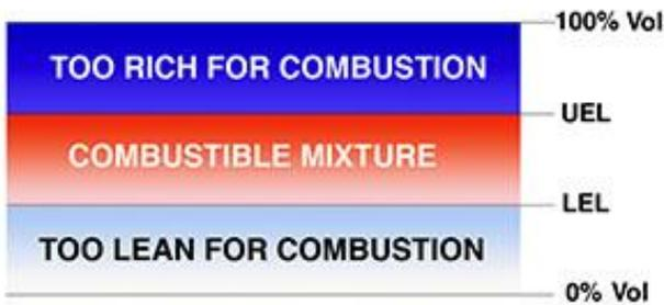
This range is defined by the lower explosive limit (LEL) and upper explosive limit (UEL) and differs for each flammable gas. At concentrations below the LEL, the mixture is too lean (insufficient fuel with respect to oxygen) to sustain combustion, and at concentrations above the UEL, the mixture is too rich (too much fuel with respect to oxygen) to sustain combustion.
