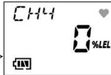
After air calibration is successfully completed, it automatically returns to the detection mode.
