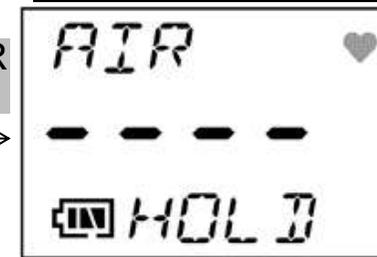
Pressing the MODE button or performing no operations for more than 20 seconds returns the gas monitor back to the detection mode.
